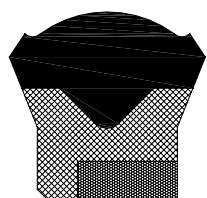
**TEOL 1A (S24)** Similar to TEOL/1 with an anti extrusion synthetic resin ring.
