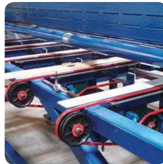
Wood panel conveyor using PowerMax Round Idlers and Eagle Red 90 belting.
