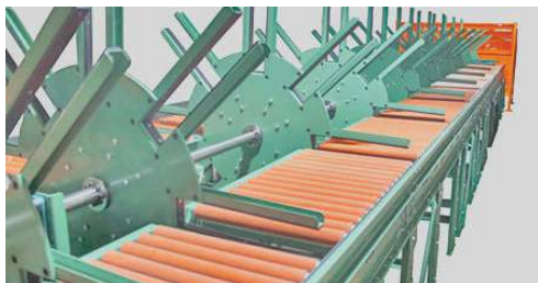
B-LOC Compression Hubs mounting transfer wheels to the shaft of a 12-strand rollover conveyor.
