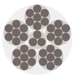
Figure 1.5.2: Tensile reinforcement structure  $3 + 5 \times 7$  in cross profile
