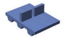
Figure 6.5.4: Rectangular cleats, arranged in series
