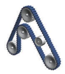
Figure 3.2.2: Multi-pulley drive with inside, smooth cylindrical pulley
