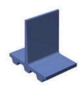
Figure 6.5.5: Triangular cleat with rounded head
