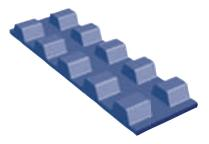
Figure 6.6.4: Longitudinal groove in tooth system
