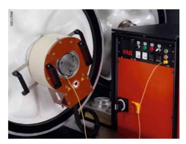
Figure 3 Rigid inductor in the dismounting of wheelset bearings
