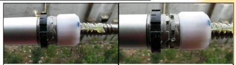
The "free-wheeling push only" nut system when the system is extending
