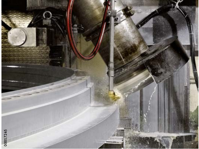
Figure 7 Regrinding of large size bearing ring
