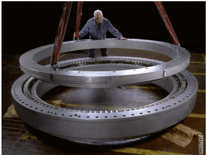
Figure 9 Mounting of a new rolling bearing ring
